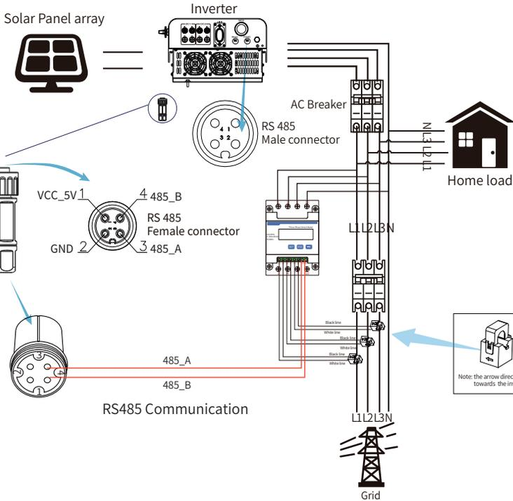
Pic 7.14 Connection diagram of CHNT meter
