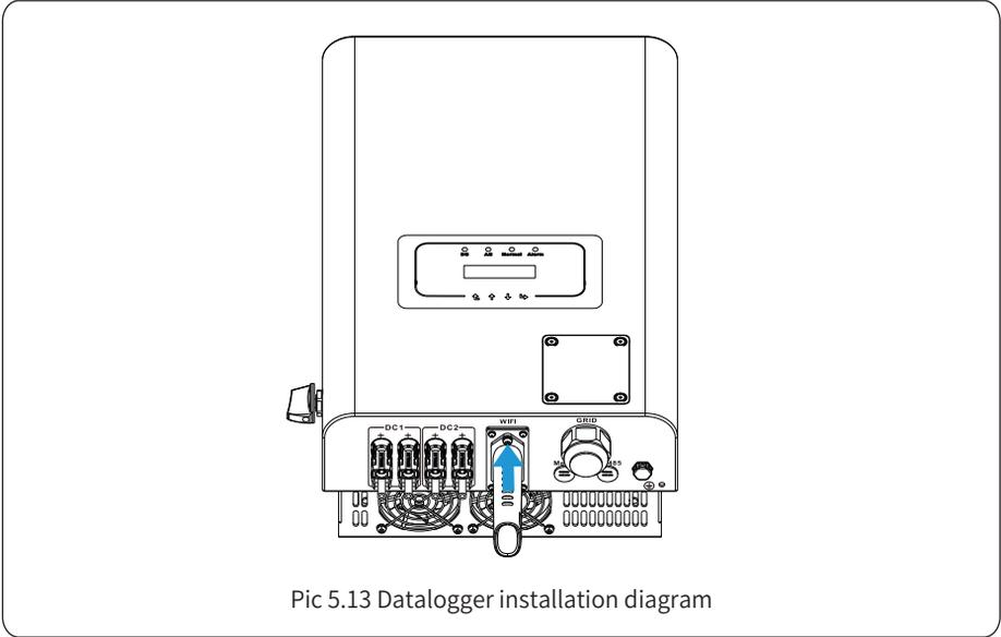
Pic 5.13 Datalogger installation diagram
