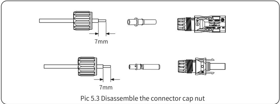
Pic 5.3 Disassemble the connector cap nut
