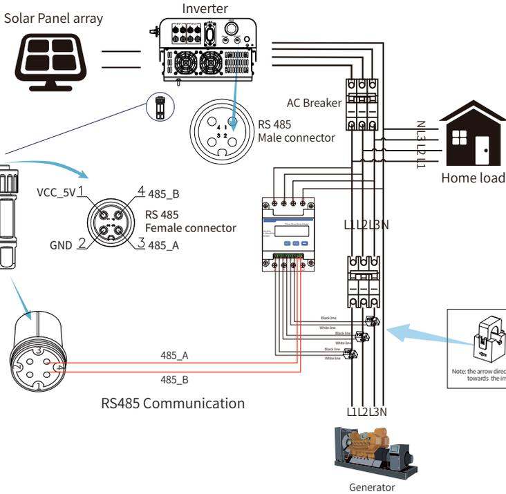
Pic 7.14 Connection diagram of CHNT meter
