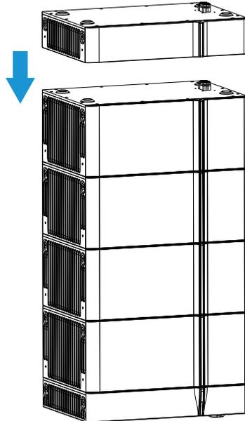
4. Finally, install the high voltage box to the top layer of the battery module.
