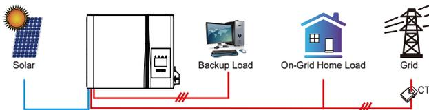
**Solar Sell:** "Solar sell" is for Zero export to load or Zero export to CT: when this item is active, the surplus energy can be sold back to grid. When it is active, PV Power source priority usage is as follows: load consumption and charge battery and feed into grid.
