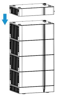
4. Finally, install the high voltage box to the top layer of the battery module.
