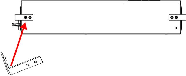
5. Use M4\*12 hex socket screws to install the box fixing plate between the base and the battery module, between the battery modules, between the battery module and the high voltage box as well.
