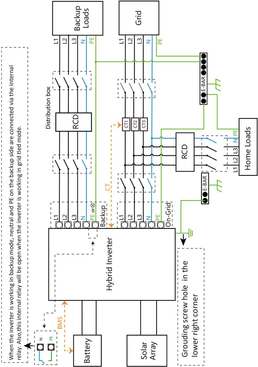
When the inverter is working in backup mode, neutral and PE on the backup side are connected via the internal relay. Also, this internal relay will be open when the inverter is working in grid tied mode.
