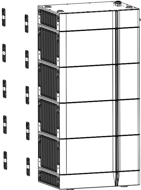
6. Place the high voltage box on one side of the wall, mark the positions of fixing holes, drill two holes in the wall with a depth of 100-110mm using the electrical drill, secure the high voltage box to the wall and install expansion bolts in the holes with a proper hammer.
