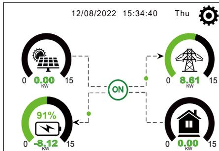
1. The icon in the center of the home screen indicates that the system is Normal operation. If it turns into "comm./F01~F64", it means the inverter has communication errors or other errors, the error message will display under this icon (F01-F64 errors, detail error info can be viewed in the System Alarms menu).
