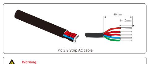
Be careful to distinguish the L1, L2,L3,N and PE of the AC cables.
