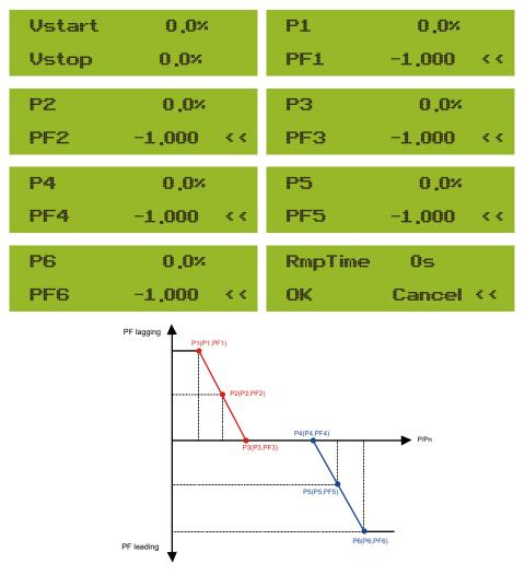
Pic 8.37 Power factor Regulation Curve in PF(P) Mode
