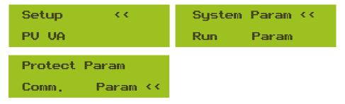
Pic 8.17 Submenus of the parameter setup
